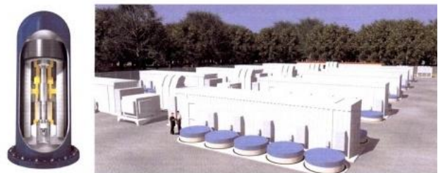
Fig. 10. An individual flywheel unit (left) and conceptual flywheel storage plant (right)
