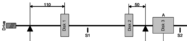
Figure 4. The rotor layout: the displacement sensors at “S1” and “S2” the actuator at “A”. The dimensions are in millimeters.
